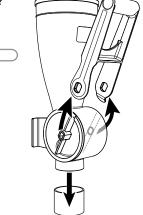
6 REMOVE CYLINDER from side of unit body.
