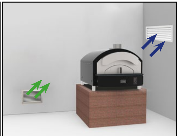
➔ NATURAL VENTILATION - S=300\text{cm}^2 ➔ NATURAL AERATION - S>100\text{cm}^2
