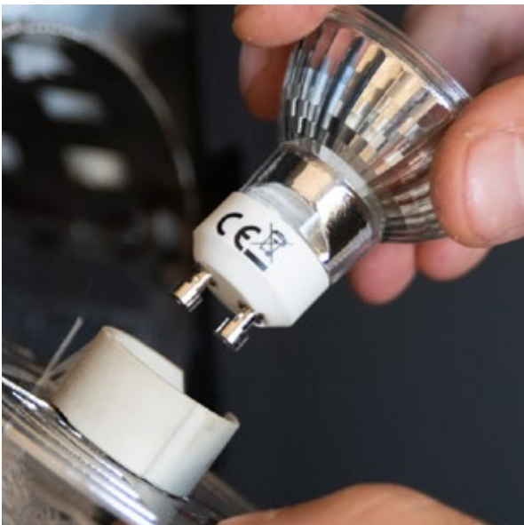
3. Unscrew the lamp and install the new one, taking care that it is not directly in contact with the internal glass
