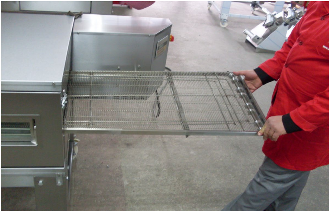
The conveyor is mounted inside the machine as shown in the picture.
