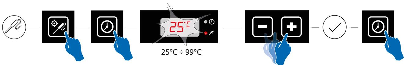
You can press button **14** again to return to timed cooking mode and then press it again to return to core probe cooking mode. But every time the cooking type is changed, the time and core probe temperature parameters are reset to their default values.
