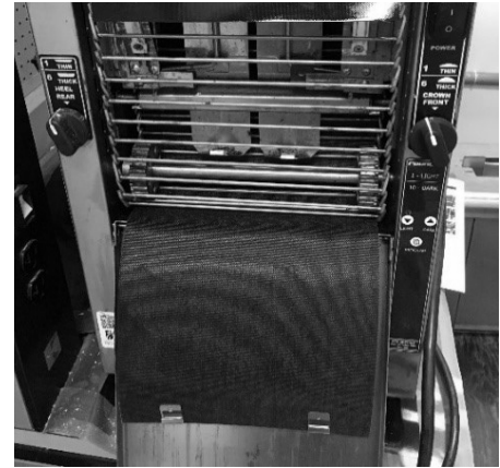
Figure 13. Remove Belt Wraps
