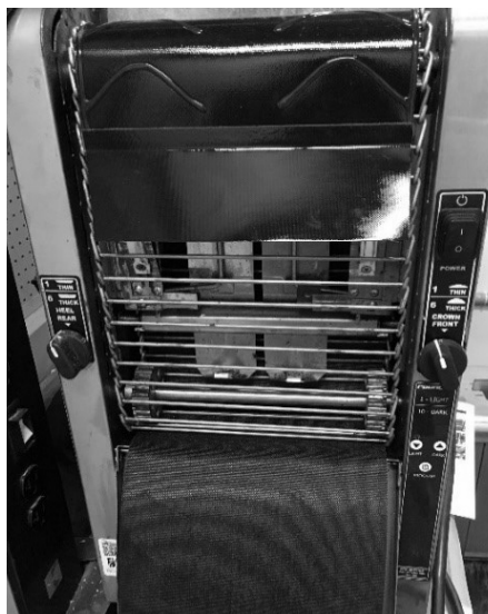
Figure 23. Remove belt wraps
