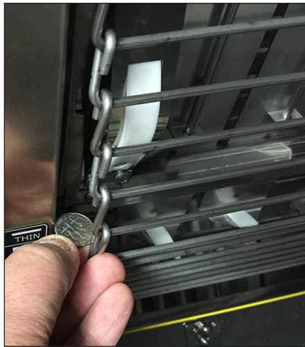
Figure 15. Measure with Dime coin
