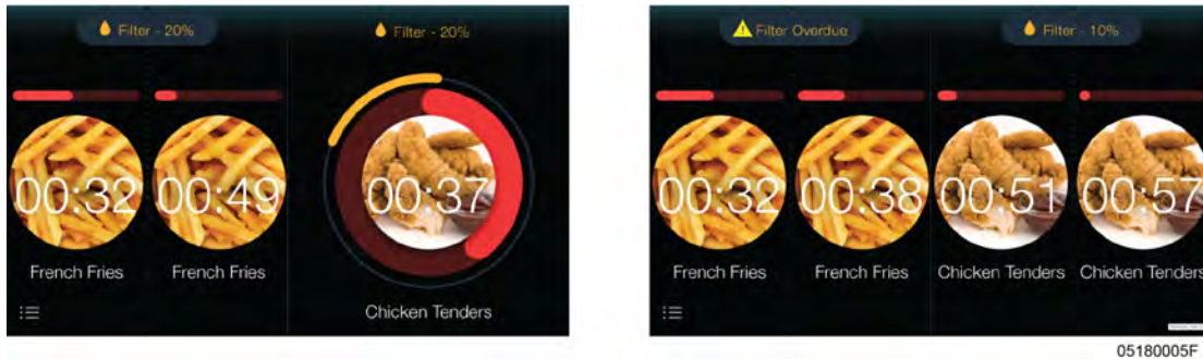
Figure 4-10 3 and 4 timer operation
