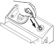
4. Replace the switch cover and secure by screwing clockwise.
