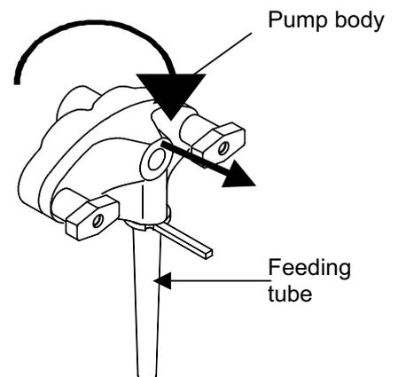
**step 9****Drain rinse water from hopper and cylinder**
