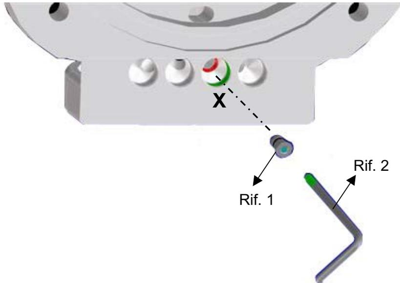
In case you are using only 3 syrup flavours, you should close the hole of the front lid using the tap ref. 1 delivered with the accessories.
