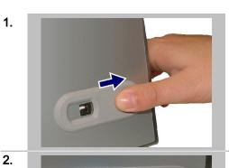
Slide the sliding cover on the USB port to the right.
