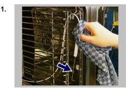
Slide the core temperature probe into the holder.
